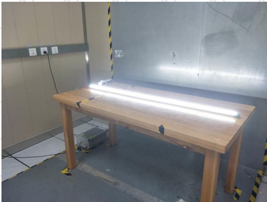
Photo 2 Conducted Emission Test
