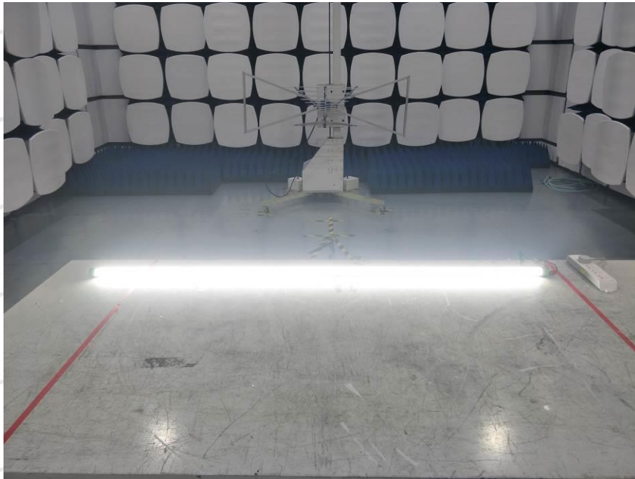
Photo 1 Radiated Emission Test
